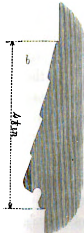
Second Set-off of Buttress.
